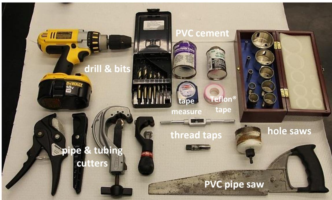
**Figure 13.** Tools typically needed to construct experimental setups. Most can be found at the local hardware store. Some like diamond-coated hole saws and plastic-specific drill bits may need to be ordered (e.g., [www.mcmaster.com](http://www.mcmaster.com)). Other tools sometimes used but not shown here are a circular saw (for cutting acrylic sheets or wood) and a Dremel® rotary tool (for cutting, grinding, and sanding).
