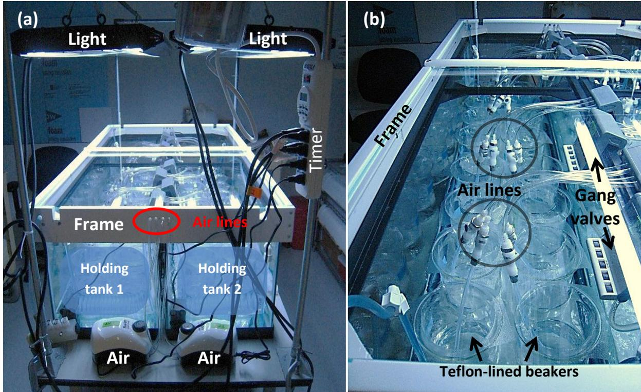
**Figure 44.** a) Side overview of chemical dosing system. Treatments are divided evenly between two holding tanks. b) Closeup side view of dosing system. Gang valves regulate the air flow in each experimental unit.
