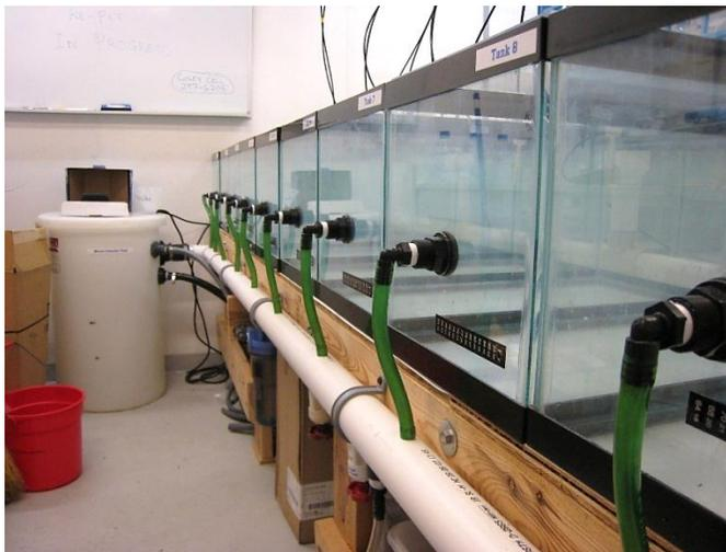
**Figure 19.** Waste seawater can drain through bulkheads and be collected in a central waste container where it can be decontaminated prior to disposal. Photo of a toxicology dosing system at the Hollings Marine Laboratory, Charleston, SC.
