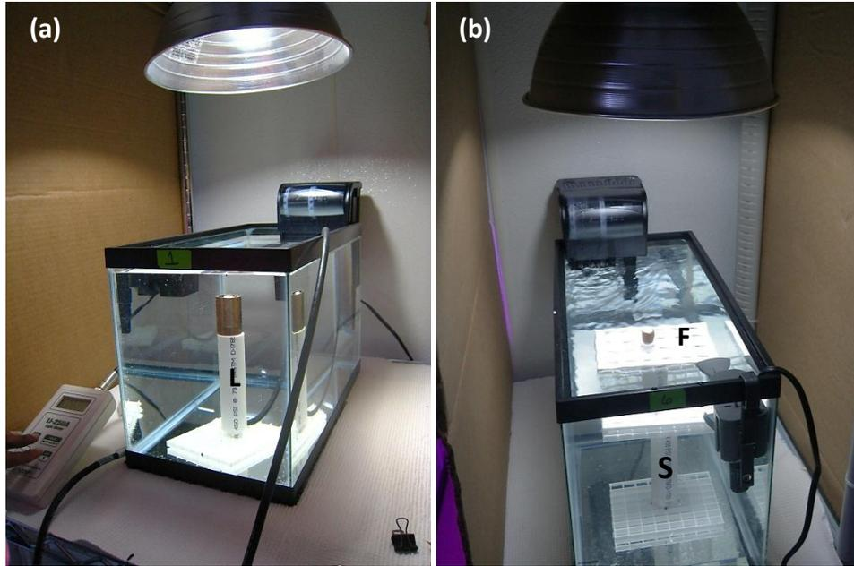
**Figure 41.** **a)** Each light is standardized to  $100 \mu\text{mol}/\text{m}^2/\text{s}$  using an LI-192 underwater light sensor (LI-COR®) mounted on a PVC stand (L). **b)** The single coral fragment (F) is centered in the middle of the tank directly under the light source at a specific height on a PVC stand (S).
