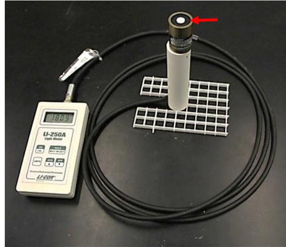
**Figure 11.** Light meter and sensor used to measure photosynthetically active radiation directly above the sensor (**arrow**). The sensor has been positioned on a stand constructed from PVC pipe and plastic egg crate material to keep the sensor stable and at a specific height in the water column.
