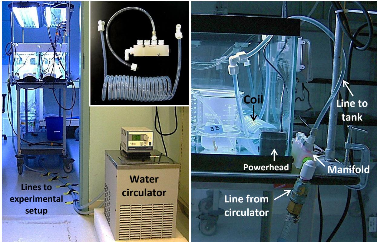
**Figure 46.** Water recirculation system for regulating temperature in the chemical dosing system. A temperature controlled water circulator pumps fresh water through a manifold and coils (**inset**) placed in each water bath. Small powerheads ensure evenly distributed water temperatures.
