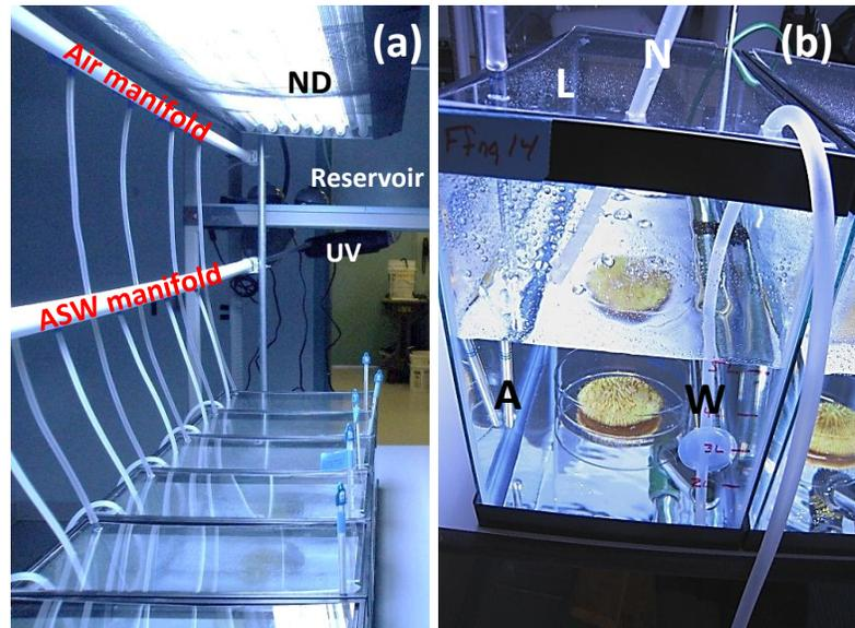
**Figure 39.** a) Side view of biological dosing setup. Neutral density shade cloth (ND) standardizes the light intensity across all the experimental tanks. b) Close-up of individual experimental tank. The air line (A), new ASW line (N), and waste siphon tube (W) enter the tank through holes drilled into the lid (L).
