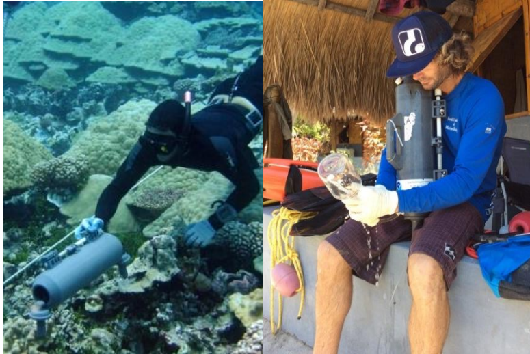
Figure 21. A NOAA-CREP SCUBA diver collecting a water sample at the reef using a Niskin bottle ( left ). NOAA-CREP field personnel transferring a water sample from a Niskin bottle to a glass bottle for later dissolved inorganic carbon and total alkalinity analysis ( right ).
