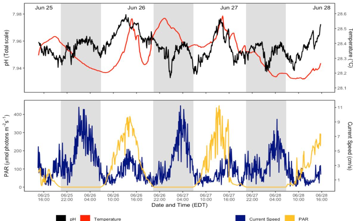
**Figure 3:** Bird Key Reef (15m) diurnal suite monitoring from June 25th to 28th. Top panel: pH and temperature from SeaFET. Bottom panel: Photosynthetically Available Radiation (PAR) and current speed from EcoPAR and Tiltmeter. Grey blocks denote nighttime throughout the sequence of the plot. Instruments measured parameters every 5 minutes over 72 hours.
