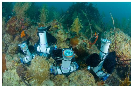
**Figure 3:** Submerged Automated Samplers (SAS) deployed to collect water samples every 3 hours.
