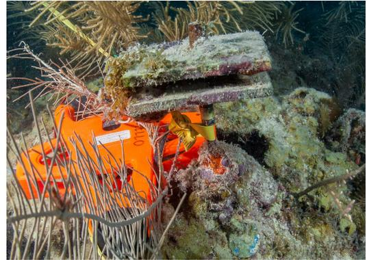
**Figure 7:** CAU and BMU pair before retrieval after being deployed for three years. CAUs are two parallel PVC plates to quantify settled accretors. BMU is mounted coral skeleton installed at the base of the metal stake and has been encrusted.
