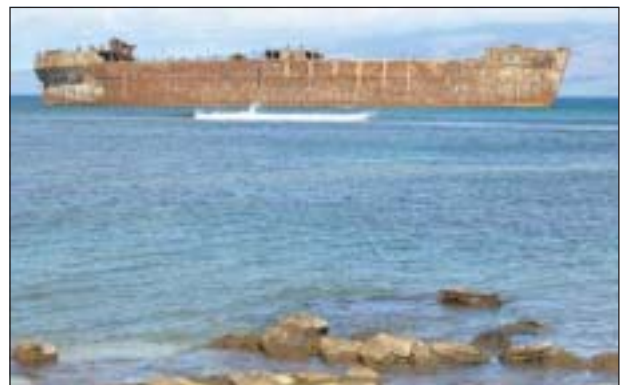
Figure 239. This U.S. Navy steel-reinforced concrete vessel has been hard aground off Shipwreck Beach, Lanai since the 1950s (Photo: Hans van Tillburg).
